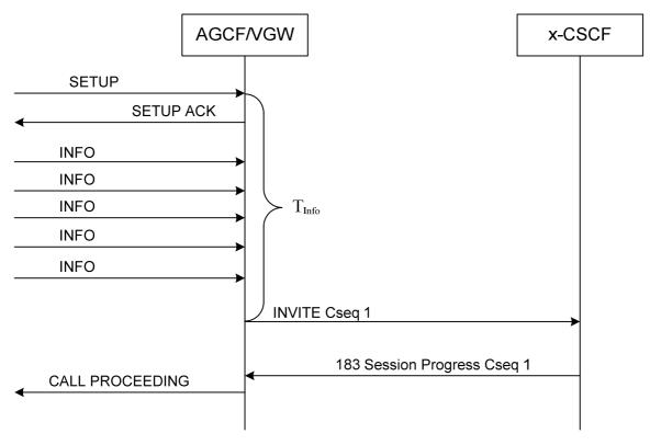
Figure D.1.1.3-1: Overlap with  $\mathrm{T}_{\mathrm{info}}$  Timer- no transaction is pending
