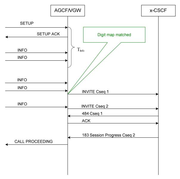
Figure D.1.1.3-5: Overlap with digit map and  $\rm T_{info}$  timer digit map matched after  $\rm T_{info}$  expiry
