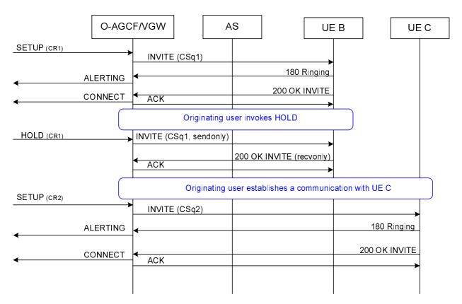
Figure G.2-1: Basic procedure and remote user is set on HOLD
