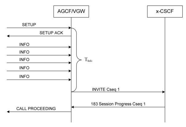
Figure D.2.1.2-1: Overlap with  $\rm T_{info}$  Timer - no transaction is pending
