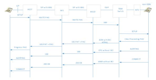
Figure H-4: Interworking situation IMS to TDM, an ISDN (PES) user is calling an ISDN user with an PBX which has a non-ISDN access
