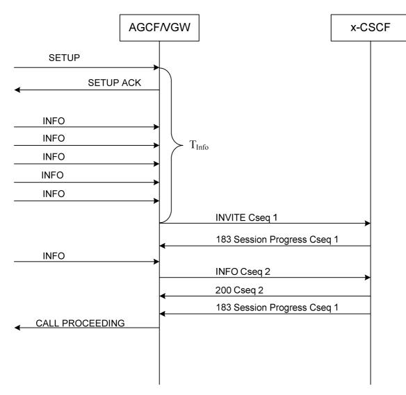
Figure D.2.1.2-2: Overlap with  ${\rm T}_{\rm info}$  Timer no transaction is pending
